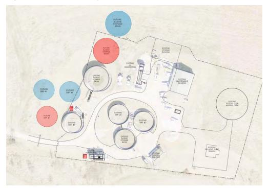
Figure 7-8. WWTP Site Layout for Phase II Expansion
