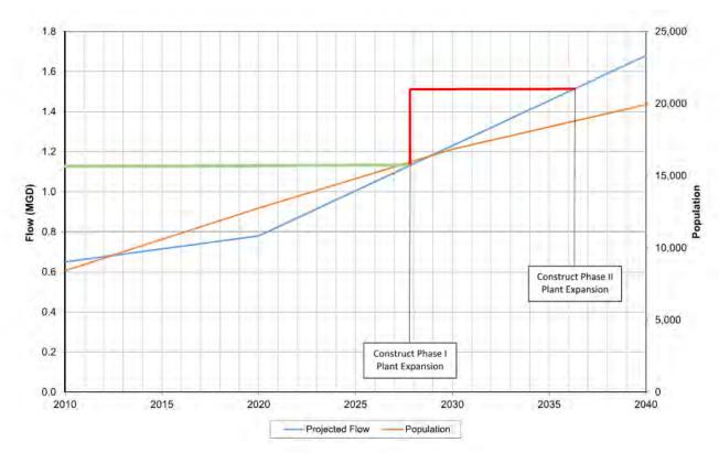
Figure 7-9. WWTP Facility Phasing Using Future Development
