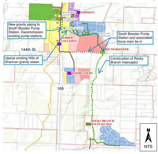
Figure 6-4. Rocky Branch Interceptor and South Booster Pump Station Projects
